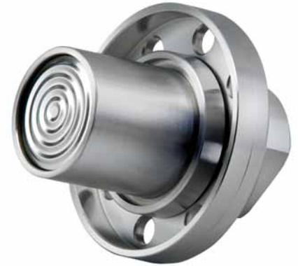
Diaphragm seals are designed to isolate the sensing element of pressure gauges and pressure switches from process fluids which may be corrosive, viscous, sedimentous and/or with a high temperature. The diaphragm is welded to the upper body, to ensure separation of filling fluid from process medium. The "in-line" diaphragm position enables deep cleaning of their surfaces. Flange clamping with metallic sealing guarantees the system against leakage at high process fluid temperatures and pressures.
